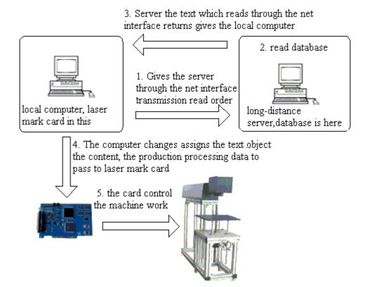
Figure 4-42: TCP/IP communication flow chart
