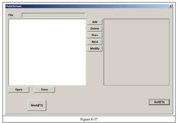
**Add:** Add .ezd files. The dialog box pops up as Figure 8-38 after click "add" button. Setting I/O control conditional for files, and automatically mark files when board accept the IO signal in mark status.
