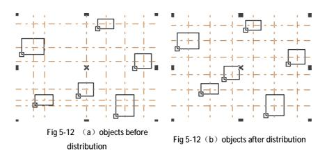
Before 'distribution' (fig 5-12a), the distance between the center of each object is different, and after 'distribution', distance between the center of each object is the same(fig 5-12b).
