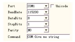
Figure 4-43 Serial communication parameters
