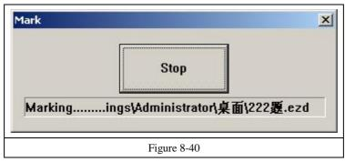
If must the accepting signals be pulse signals, should set IO port that doesn't show in figure 8-38 in start mark IO. For example, port 0-3 show in figure 8-38, should set other port in start mark IO, as port 6. Press mark, then pop up figure 8-41. When the board accept the start mark IO and setting IO control conditional at the same time, the files will be marked only one time.
