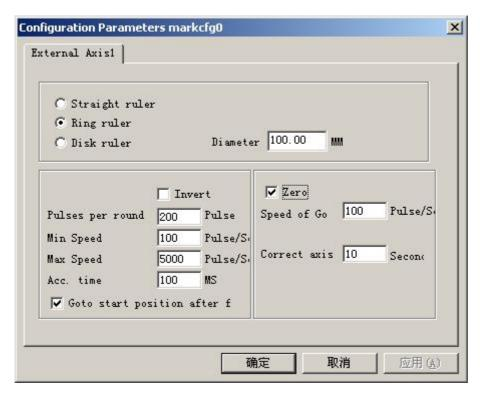
Figure 8-25 configuration parameters of expansion axis
