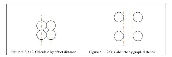
**Calculate by graph distance:** The space of the graphs is calculated by graph distance. (Figure 5-3(b))
