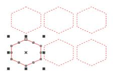
Figure 2-14 Array (X=3, Y=2)
