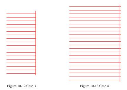
Different manufacturers use different Laser sources and scanner(gavlo), so the performances are also different. Sometimes when however users modify the **End TC**, the hatch-lines and the border cannot be superposed. Here users need to set the **End Compensate** (Values from 0.05 to 0.25). But this may cause the 4th case: the hatch-lines are beyond the border, as Figure 10-13 shows. Users should lower the **End Compensate** to reach the perfect result.
