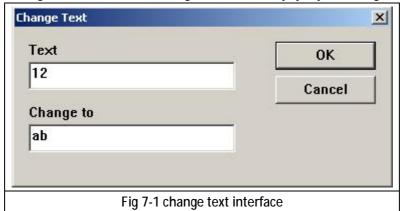
The content under 'text' is to be replaced, the content under 'change to' is that after replace. Fig 7-2b is the result after operate fig 7-2a as the method in fig 7-1.
