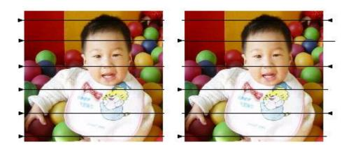
Figure 4-57 Left is unilateral scan; right is bidirectional.
