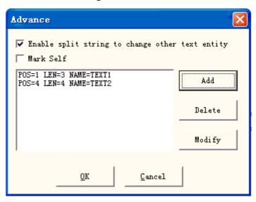
Figure 4-50-d The result add split character string 6. Click "Mark" then the dialog box will be displayed shown as Figure 4-50-e, the user use bar code scanning gun scanning the ticket's bar code, the system will put the series number division to inside
