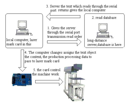
Figure 4-44 Serial communication flow chart
