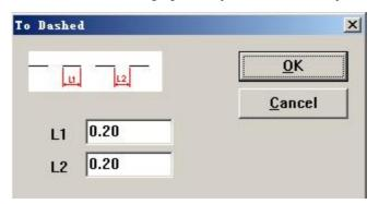
Fig 3-12 turn vector graphics into dashed object Use could set the length of the line and the distance between two lines
